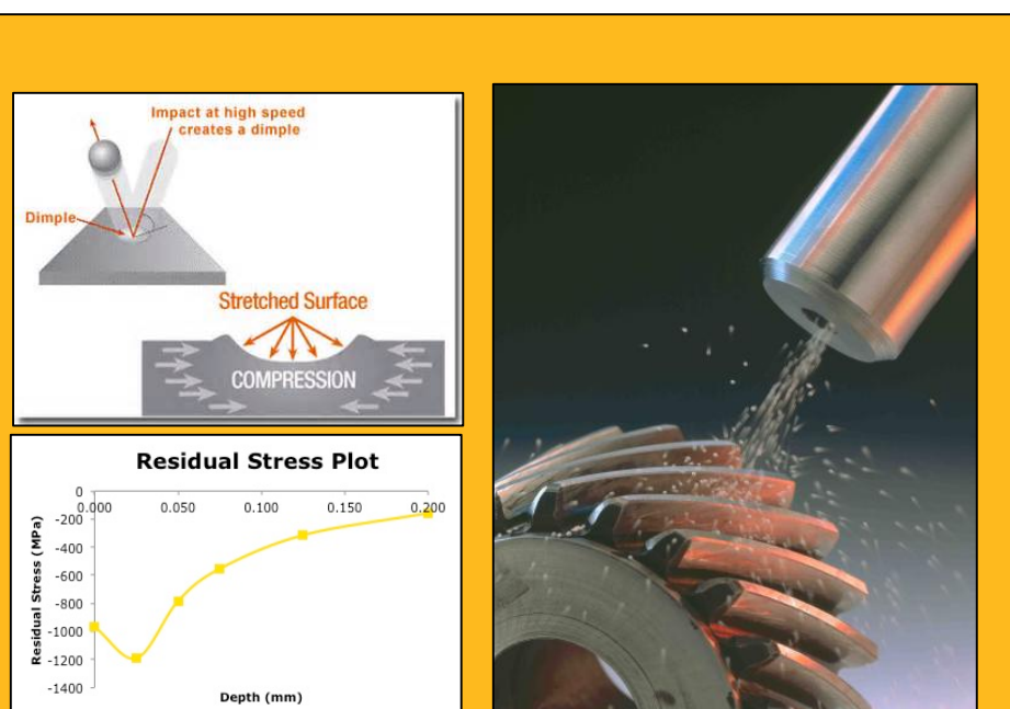
Figure 5: The shot peening process imparts additional compressive stresses into the gear surface. The shot media is usually in the form of small steel balls with a hardness greater than that of the material. A desirable post shot peening stress profile is shown on the left.
